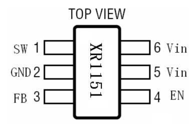
Figure 2. PIN Configuration
