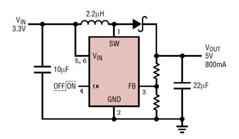
Figure 1. Typical Application Circuit
